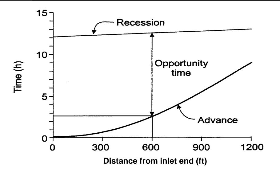
Figure 10.2. Advance and recession curves for surface irrigation.
