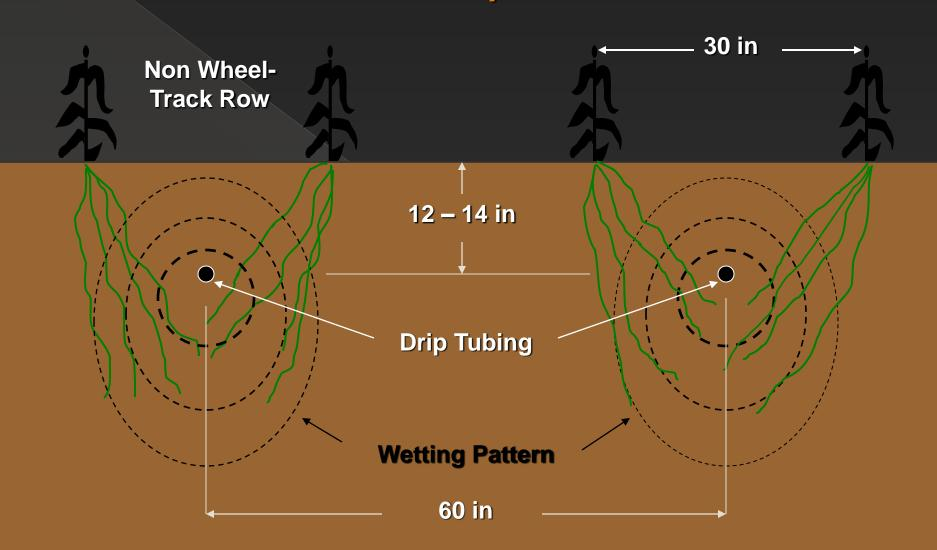
60-inch dripline spacing is satisfactory on silt loam & clay loam soils
