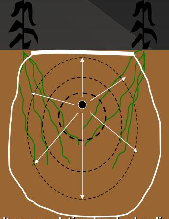
Salt accumulation leached radially outward from drip tubing
