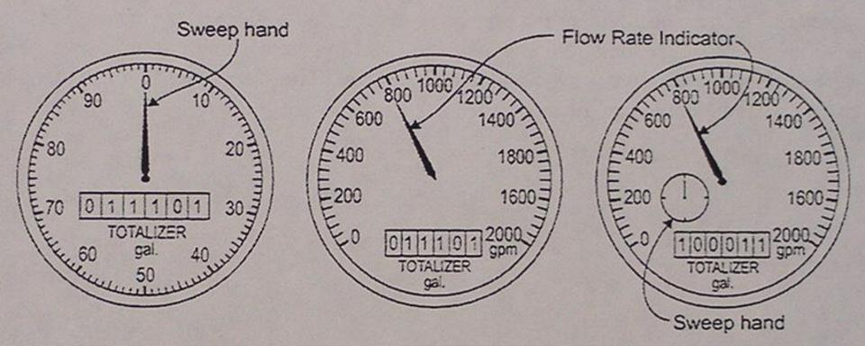
Figure 3.5. Options available for registers on a propeller meter.
