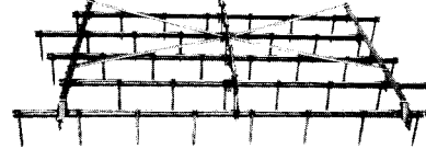
Figure 45 – Harrow—Sections, spike teeth
