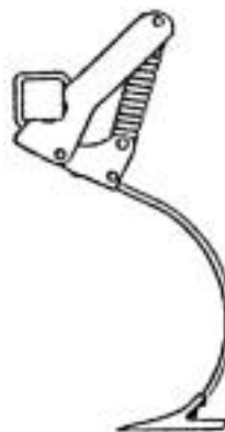
Figure 69 – Field cultivator shank—Material cross sections are usually less than 19 mm (0.75 in.) thick and of various widths—Shapes are described as 'C' shape, 'S' tines, 'K' tines, and spring tooth
