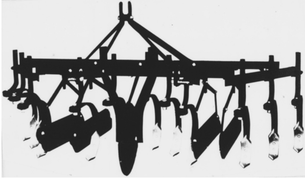
Figure 41 – Row crop cultivator—Same as Fig. 40 except two-row, rolling couler for lateral stability
