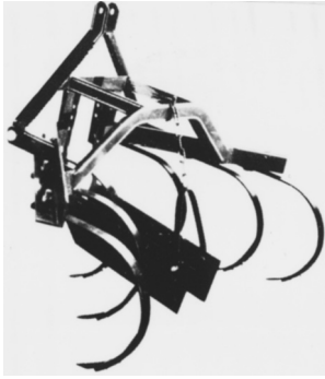
Figure 40 – Row crop cultivator—One-row, spring teeth, crop shields—Rear-mounted
