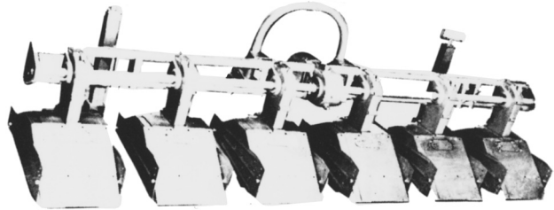
Figure 60 – Rotary tiller—Strip tiller with crop shields for row crop cultivation—Rear-mounted
