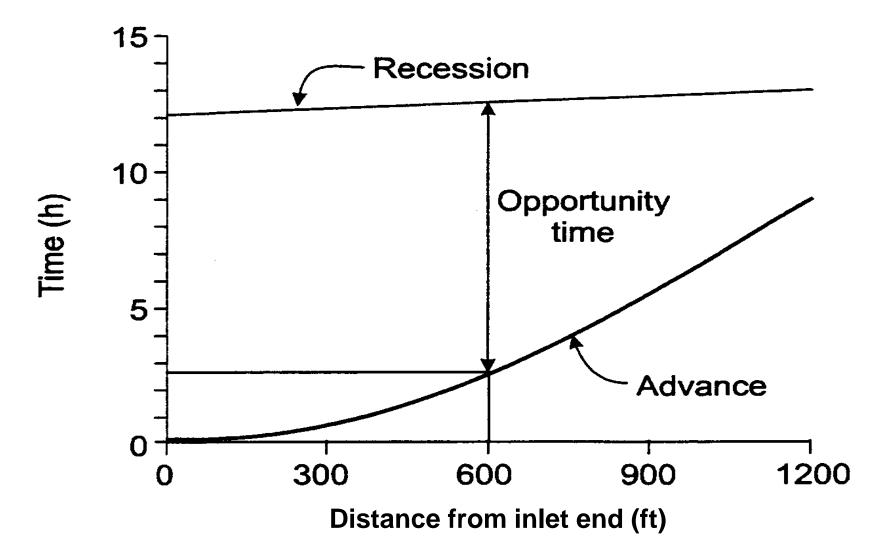
Figure 10.2. Advance and recession curves for surface irrigation.
