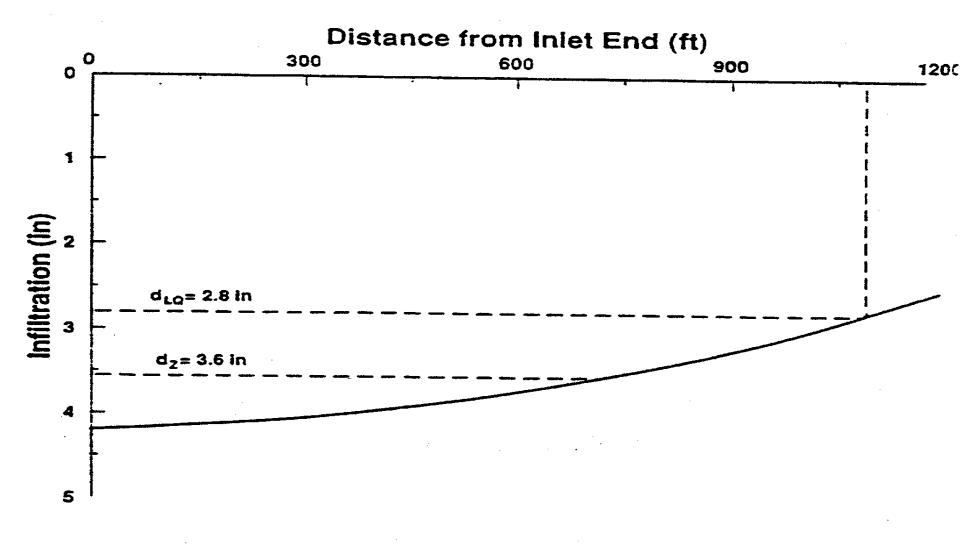
Figure 10.5. Infiltration profile.
