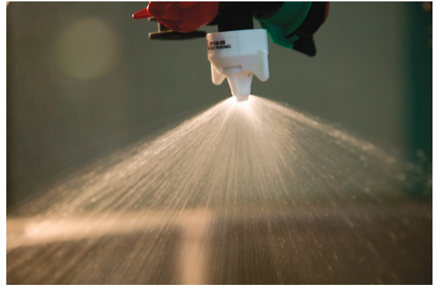
Figure 3. Different nozzles create droplet patterns used for a variety of purposes. (Refer to Table 1 for droplet size categories.)
