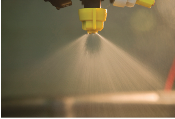
Figure 3. Different nozzles create droplet patterns used for a variety of purposes. (Refer to Table 1 for droplet size categories.)
