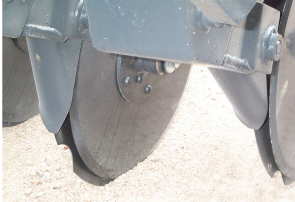
Figure 9. A double disk opener on a no-till drill with staggered disks and a notched leading blade.
