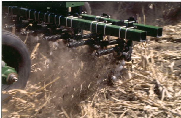
Figure 10. Tillage action of coulters on a no-till drill.
